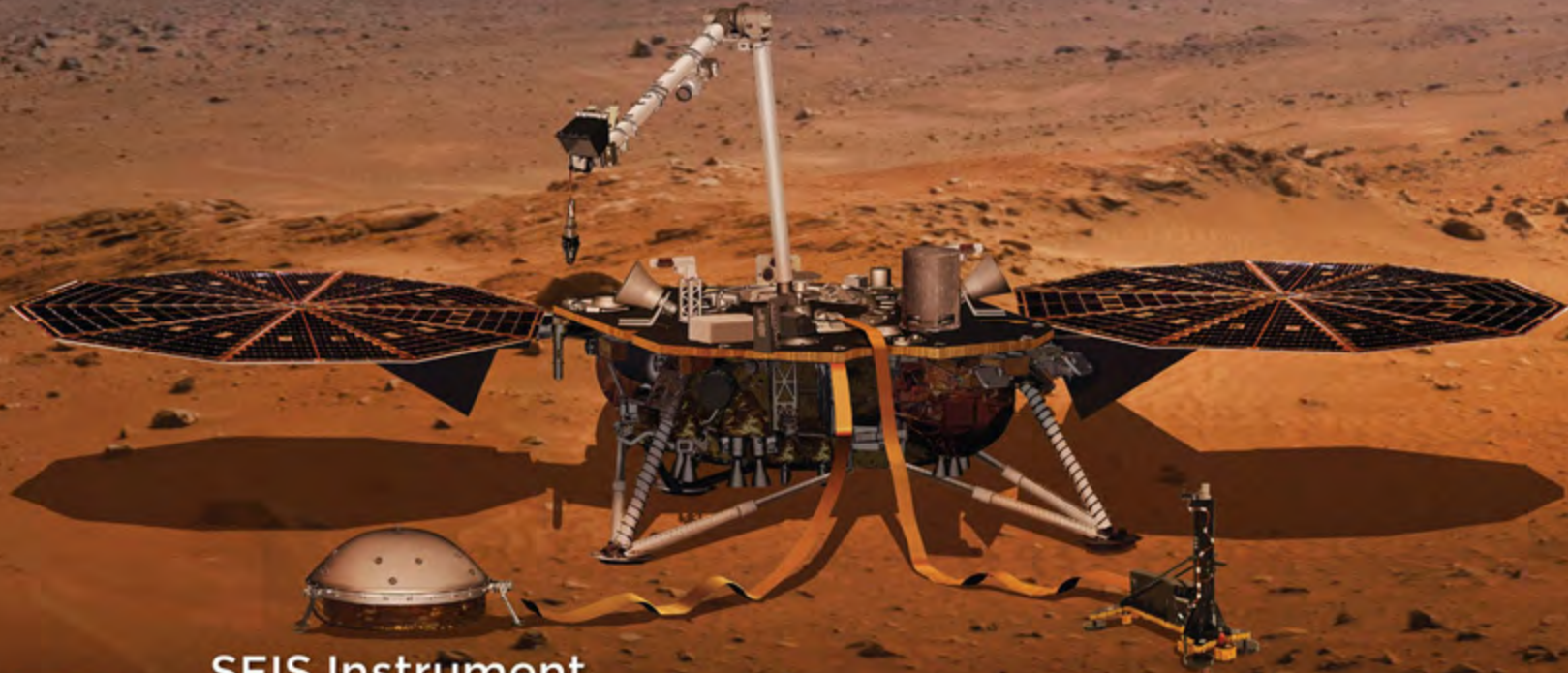
SEIS Instrument (covered with Wind & Thermal Shield)
