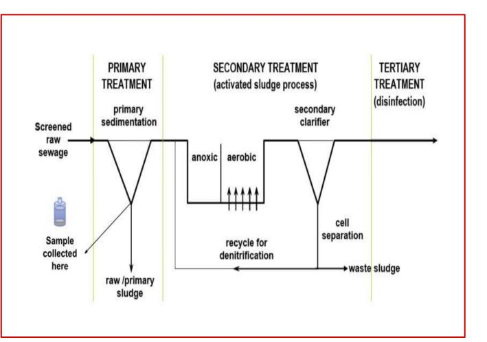
Schematic of wastewater flow at NYIT wastewater treatment plant (WWTP
